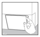
• Place a container close to the pump to collect any spillage.
